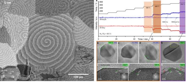
**Left:** Propagating reaction fronts observed by *in situ* SEM during  $NO_2$  hydrogenation on polycrystalline Pt. **Right:** MS data showing consumption of  $O_2$  and  $H_2O$  formation during  $H_2$  oxidation on Cu particles. Simultaneously recorded TEM images reveal oscillatory redox dynamics and co-existence of Cu and  $Cu_2O$ . More details will be provided in the talk and are available in [1] and [2].
